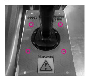
Remove the artwork plate and ligthing panel by lifting them over the top of the Joystick Controller
