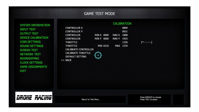
**Controller X** Shows P1 Controller X axis position **Controller Y** Shows P1 Controller Y axis position Controller Trigger Min/Max X **Shows Controller X values Shows Controller Y values** Controller Trigger Min/Max Y Throttle Min/Max X N/A Throttle Min/Max Y N/A **Calibrate Controller Executes Controller calibration routine** Revert to default values **Default Setting**
