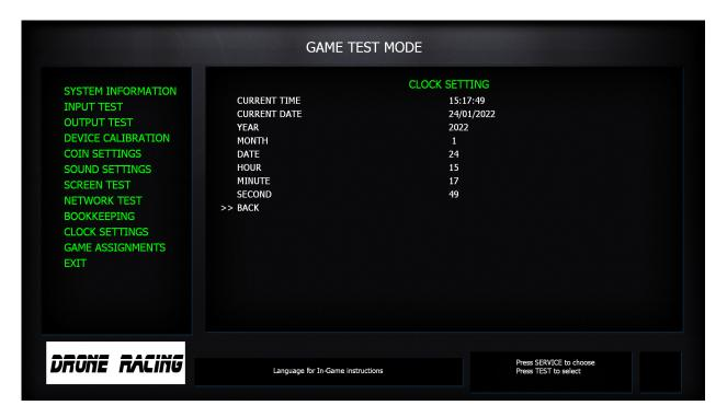
**Current Time** Displays current time **Current Date** Displays current date Year Adjusts year Month Adjusts month Date Adjusts date Hour Adjusts hour Minute Adjusts minute Second Adjusts second
