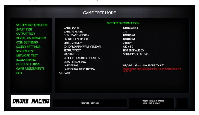
Use the Service button to cycle through the options and the Test button to select an option.
